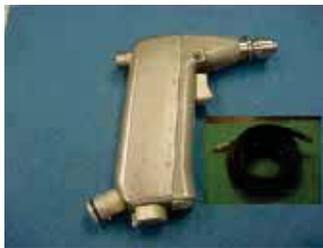
**Figure 4:** Pneumatic-powered surgical instrument with hose
